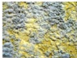
30 SULPHATE PRECIPITATION FROM TAILINGS
