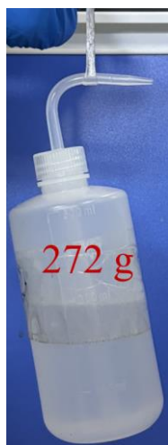
Figure S3. The picture of T_{0.3}H_{0.3} hydrogel withstood the maximum weight up to 272 g.
