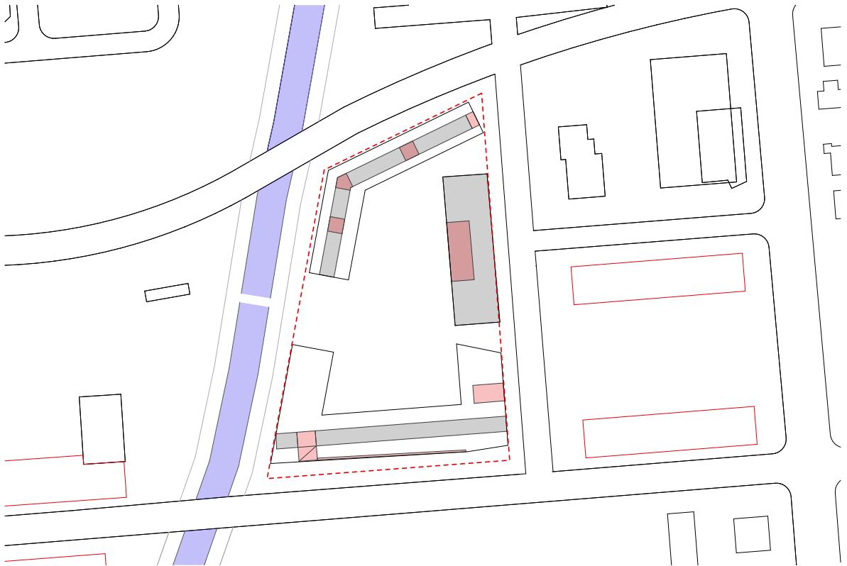
Fig 7.51 Plan Diagram illustrating service points in the building (Author, 2014).
