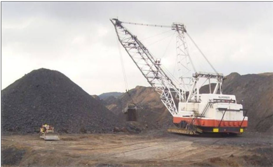
Figure 3.8: Klipspruit Colliery’s Dragline
