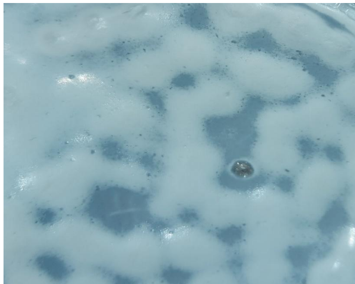
Figure 5: Agglomerations of unmodified CNFs in neat CA.
