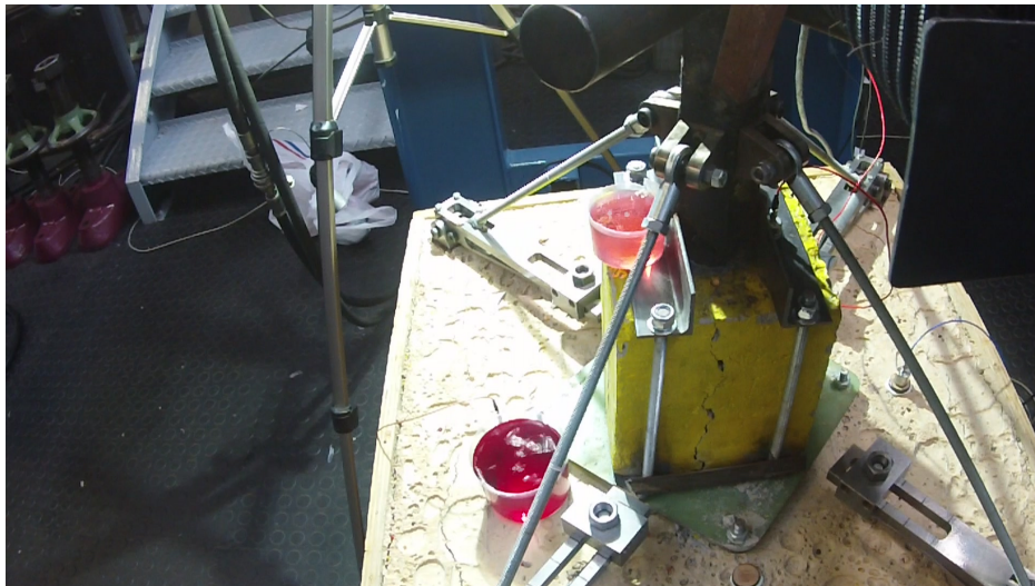
Figure 98: Tuned for 34.7 Hz antiresonance excited at 15 Hz
