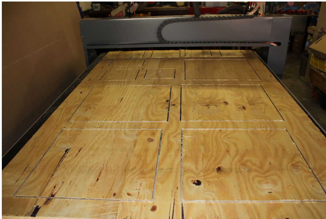
Figure 106: Routing of fuselage casting boxes using CNC router
