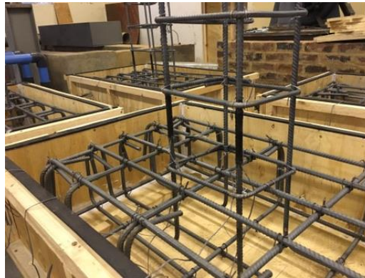
Figure 3-46 Strain gauges fixed to reinforcing bars
