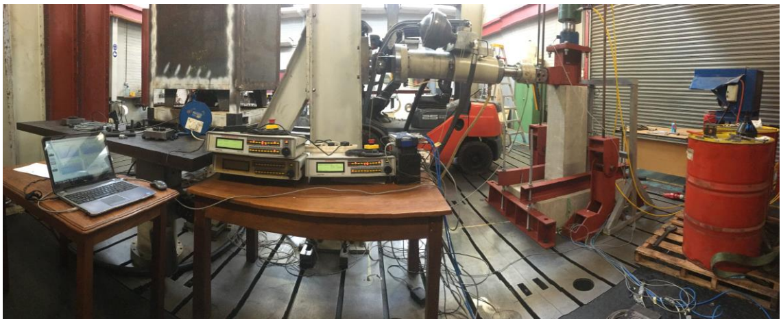
Figure 3-47 Pseudo-dynamic analysis control system
