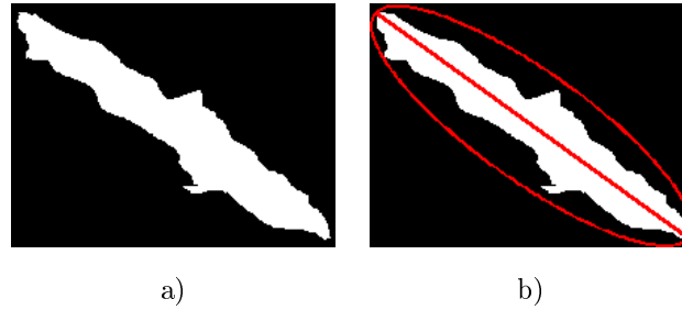
Figure 2.27: Illustration of the calculation of length. a) An image object. b) The major axis of the smallest ellipse containing the image object is the length.
