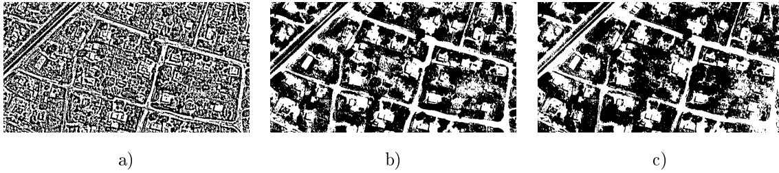
Figure 3.7: The results of various block size parameters for mean thresholding. Block sizes of 11, 71 and 501 are demonstrated in a), b) and c) respectively.
