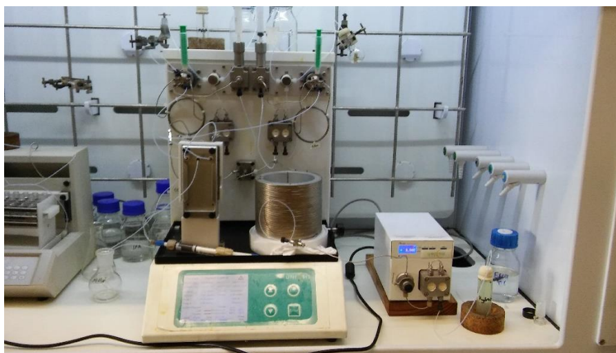
Figure 6.2: Photo of flow reactor setup for continuous multistep flow synthesis of celecoxib ( 27 ).
