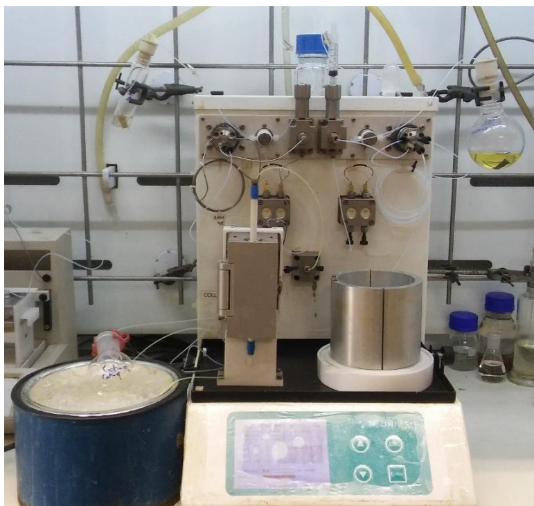
Figure 4.1: Photo of flow reactor setup for flow synthesis of aryl diazonium tetrafluoroborate salts ( 113 ).
