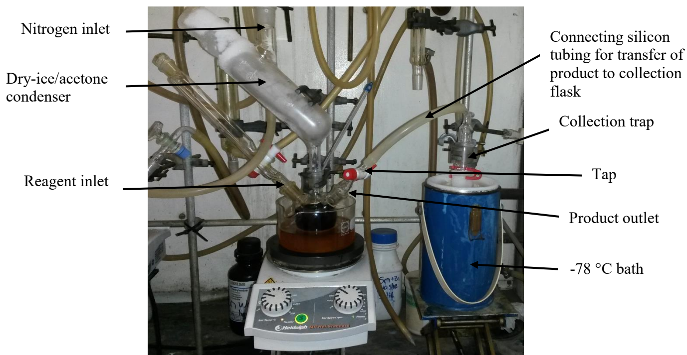
Figure 3.2: Photo of batch experimental setup for synthesis of HFBD (105).
