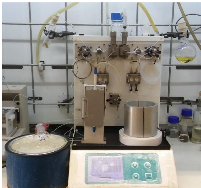
Figure 1: UniQsis FlowSyn SS reactor set-up for the synthesis of aryldiazonium tetrafluoroborates
