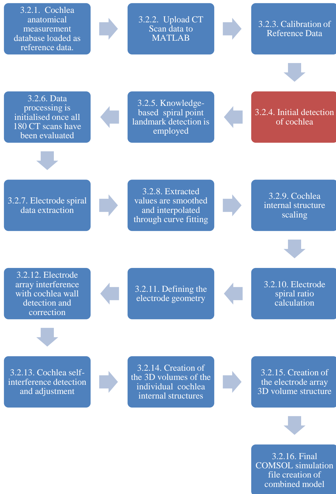
Figure 3.1 – Flow diagram of the systematic series of events followed in the KBLDA.
