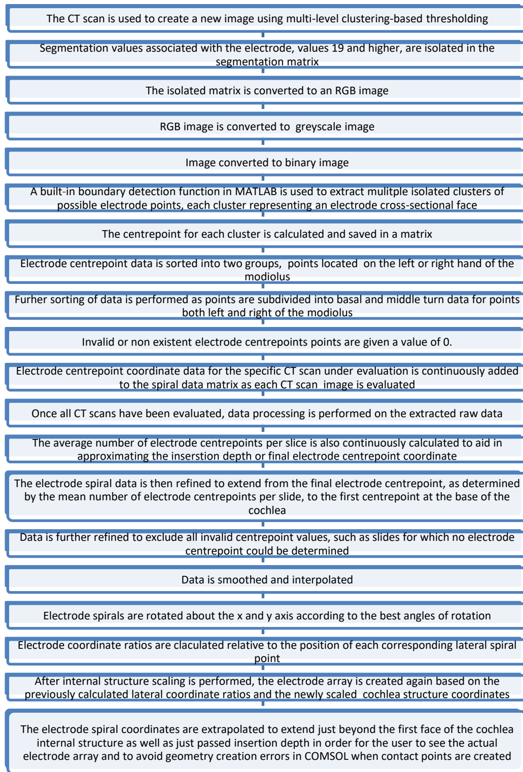
Figure 3.10 - Workflow diagram followed by the developed function to detect the electrode spiral coordinates.
