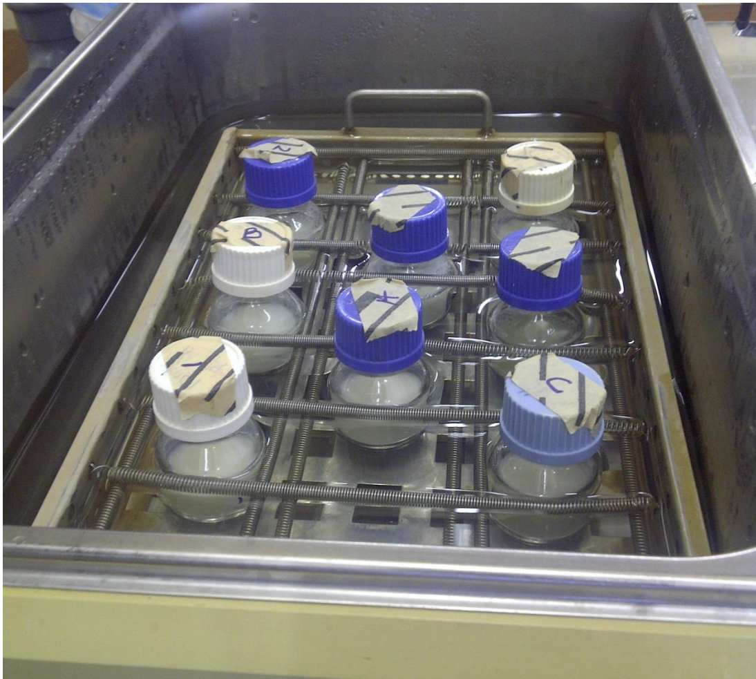
Figure 16: Schott bottles with inoculated isolated from the nozzles of ESL milk filling machines, 40ml UHT skim-milk incubated at 37°C in a shaking water-bath at 65rpm for 20h
