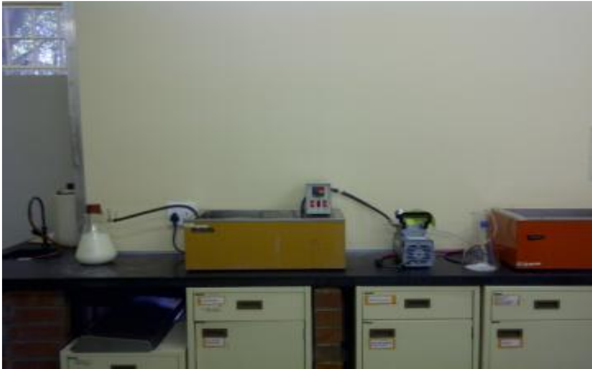
Figure 17: Laboratory biofilm reactor system used to evaluate the ability of the isolates to attach and form biofilm on the stainless steel strips
