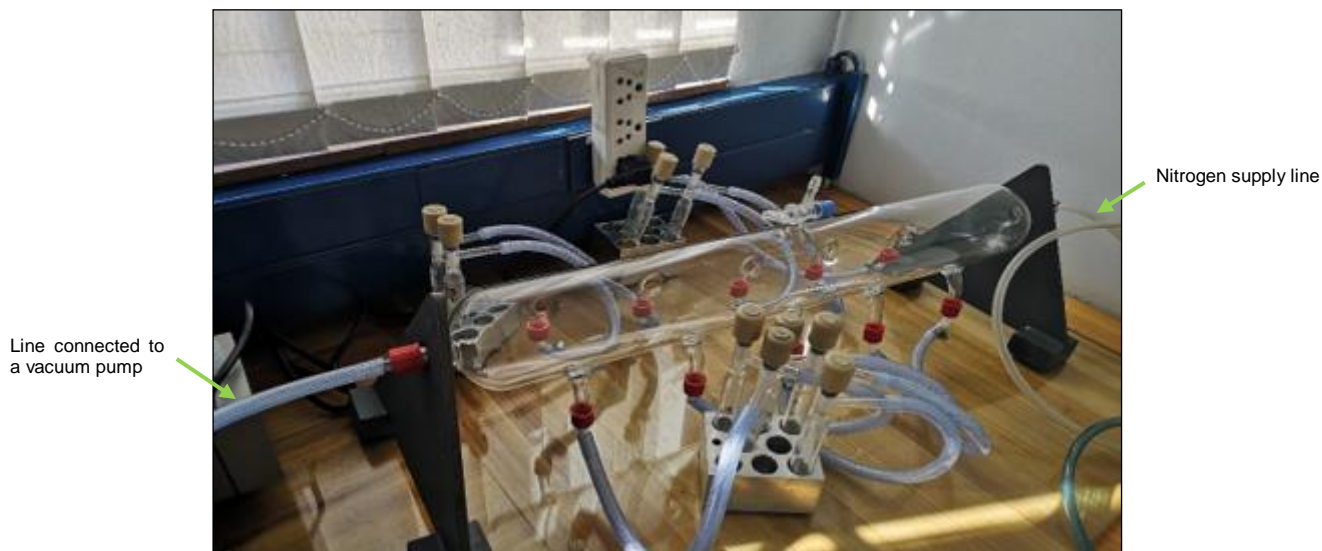
Figure 4.2. Vacuum manifold setup to purge and evacuate the hydrolysis tube headspace. The gas used for purging was nitrogen.
