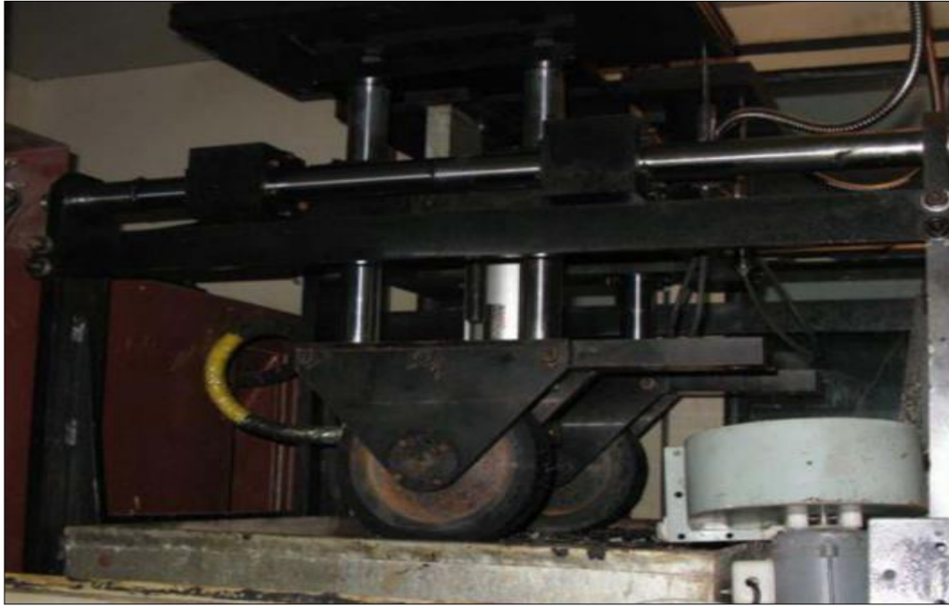
Figurer. 5-10: Wheel tracking test
