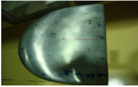
Figure 6 MAV lower wing in the test section
