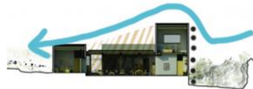
Figure 66: Section through House van der Watt indicating wind movement (Adapted by Author, from Wolff Architects (2024:online).
