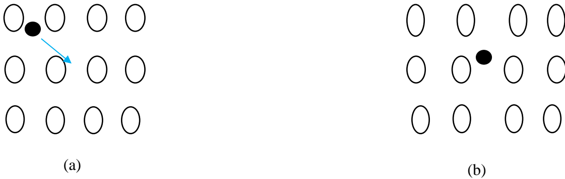
Figure 4.2: A representation of interstitial diffusion mechanism, (a) before and (b) after interstitial diffusion [6].
