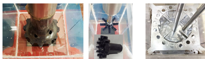
Figure 3—Impeller and stator configurations of the Denver (left and centre) and Leeds (right) laboratory cells
