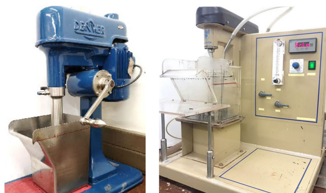
Figure 2—Photographs of Denver (left) and Leeds (right) laboratory cells at the University of Pretoria
