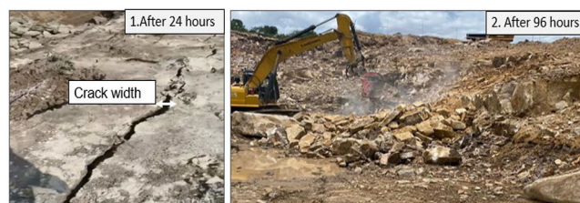
Figure 9—Fragmented rock for Trial 2
