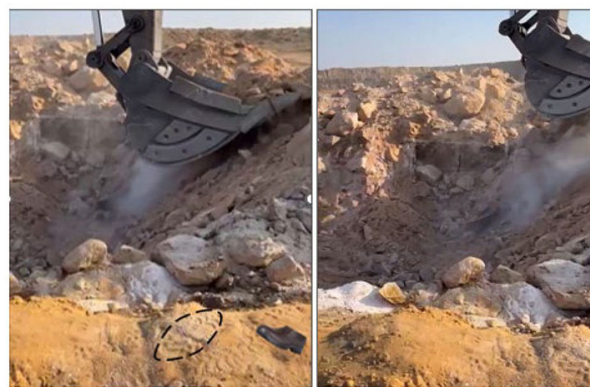
Figure 13—Fragmentation results and ease of loading the fragmented material
