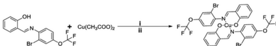
SCHEME 2. Synthesis of the complex ( \text{CuL}_2 ); i = \text{CH}_3\text{OH}/\text{CHCl}_2 ; ii = RT/4 h.
