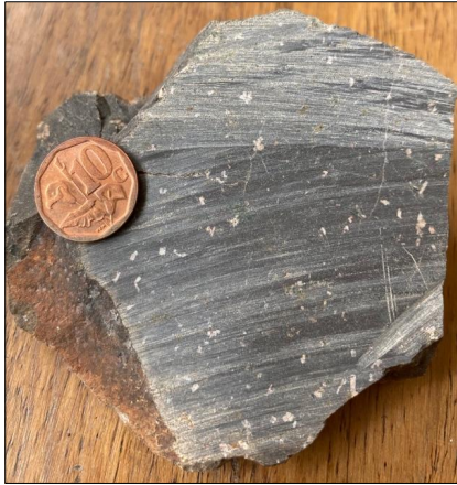
Figure 44. Hand sample of a porphyritic and dense darkly coloured rock. This rock is crystallised from a lava flow, being an andesite or dacite in composition.
