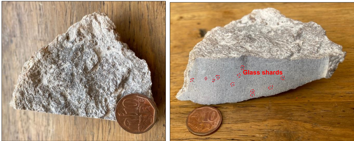
Figure 66. Hand sample of a light grey rock with a fine-grained matrix, containing glassy specks and pumice fragments. KTP 2 is a low to non-welded rhyolitic ignimbrite.
