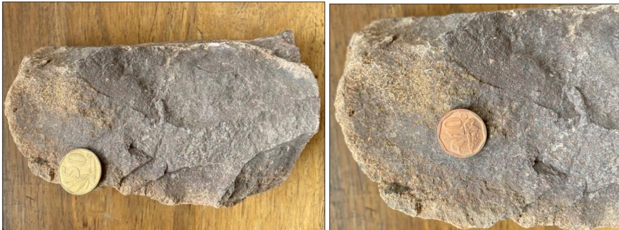
Figure 46. Hand sample of an aphanitic, lightly coloured rock of intermediate composition, such as andesitic to dacitic.
