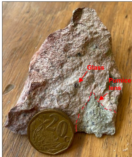
Figure 70. Hand sample of a light grey to red coloured rock with a fine crystalline matrix containing specks of glass and altered small to large pumice lenses. PYR 1B is a low to medium welded ignimbrite of rhyolitic composition.
