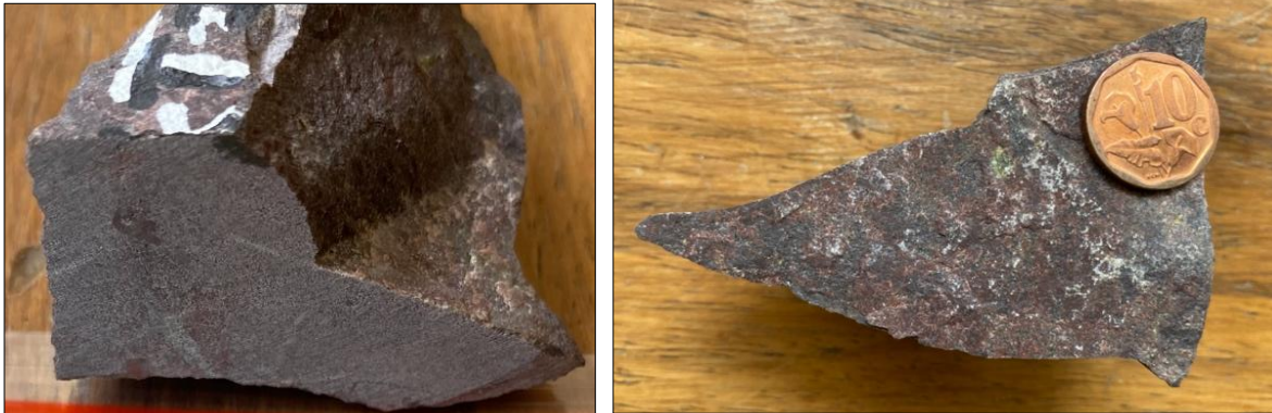
Figure 62. Hand sample of a dark, purplish rock comprising an overall aphanitic texture with sparse (1%) phenocrysts. KT 202.1 is a highly welded, lava-like ignimbrite.
