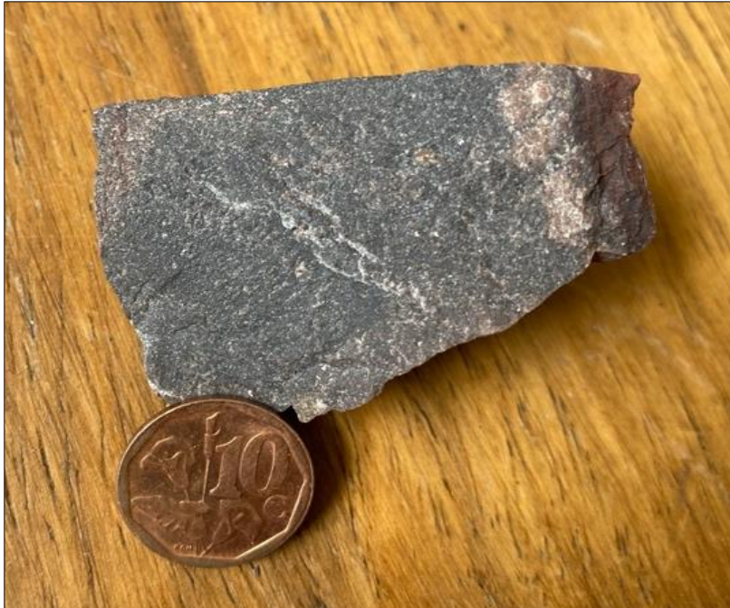
Figure 56. Hand sample of a darkly coloured, aphanitic rock, with a lava-like texture. KT 53 is a highly welded, lava-like ignimbrite of rhyolitic composition.
