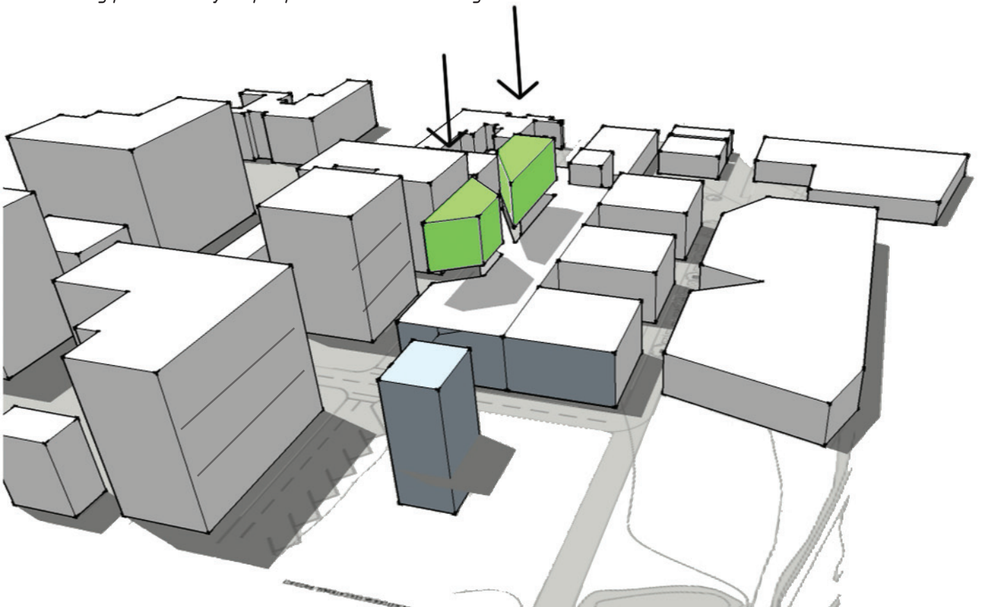
5.31 Allowing permeability to people and ventilation/light
