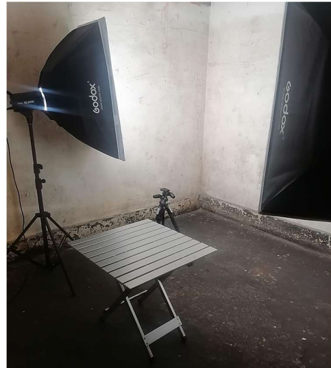
Figure 44: The camera set-up for raking lighting photography of the corner sections of the walls. photograph by author.
