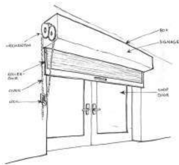
Figure 23: Parts and functions of a typical roller-shutter door in Robert Sobukwe Street
