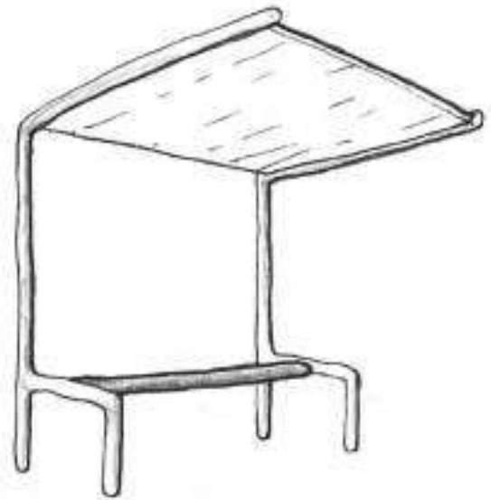
Bus top equipped with round pole to discourage loitering
