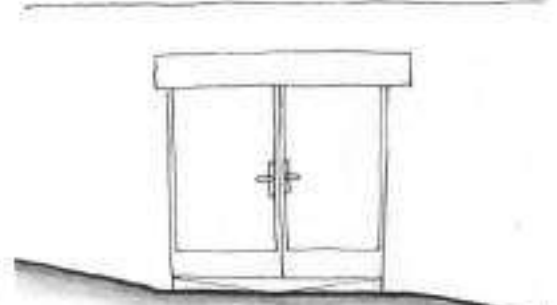
Solution: outdoor floor levelled and small ramp added
