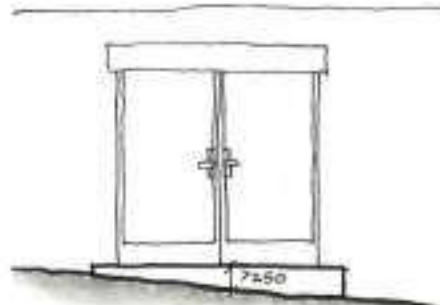
Average or centre of entrance step is too high
