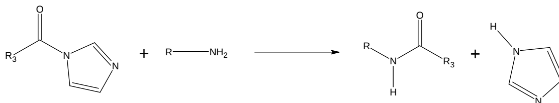
Figure 3.16 Reaction scheme for the reaction of an acyl imidazole with a primary amine. R = alkyl or aryl substituent, R 1 = CH 3 , CF 3 , C 2 F 5 or C 3 F 7 [121].
