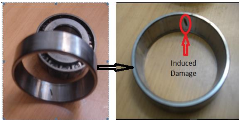
Figure 2.3, Seeded damage on outer race of a bearing.
