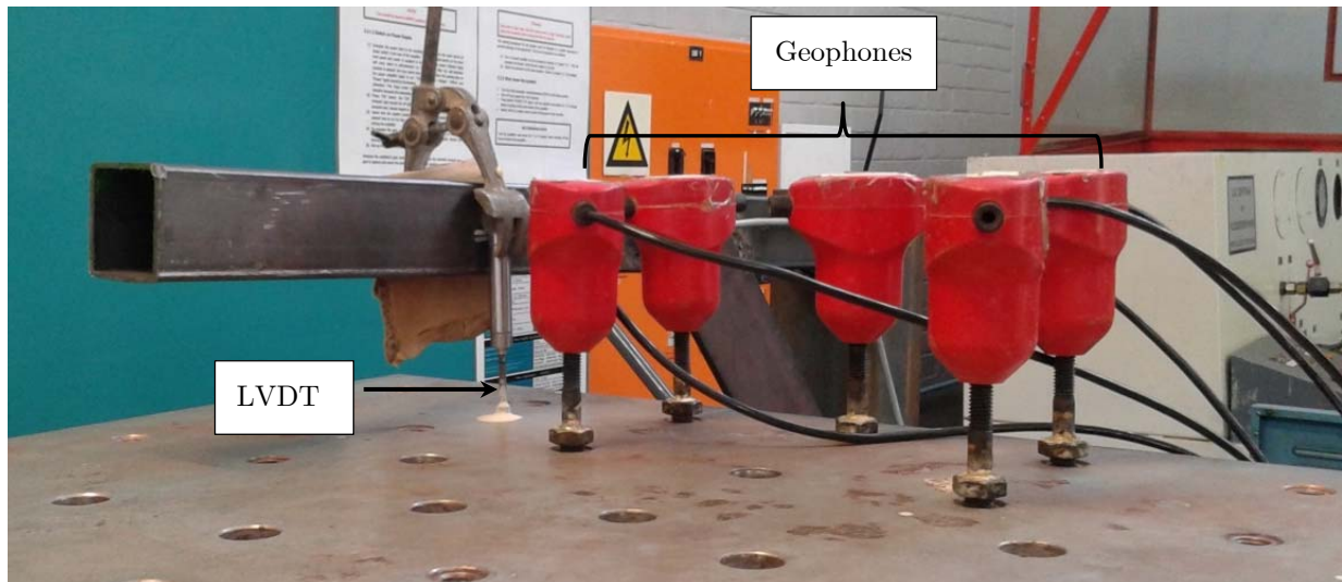
Figure 4-9: Setup adopted for geophone calibration
