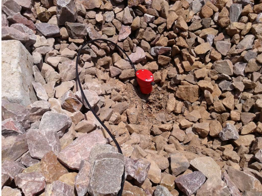
Figure 3-13: GS-11D placed on top of the subballast layer to measure vertical ground vibration
