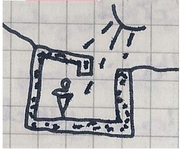
Figure 6.14 Underground structure with opening for natural sunlight [March 2009]
