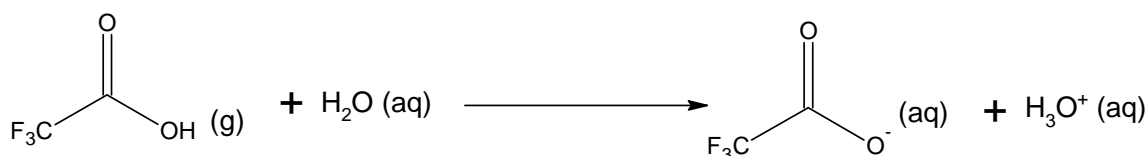
Figure 6.35 Reaction equation for the TFA acid by-product in the presence of water.
