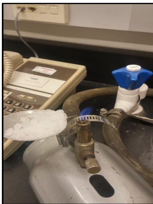
Figure 3-11: Sealing of a capillary tube containing a highly volatile component using dry ice
