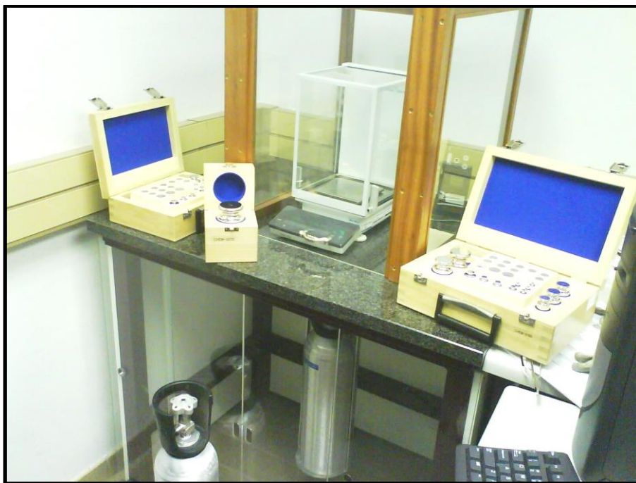
Figure 3-5: Mass comparator with suspension pan for 5 dm 3 cylinders
