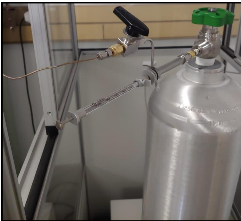
Figure 3-15: Addition of BTEX into the cylinder using KRIS heating syringe block
