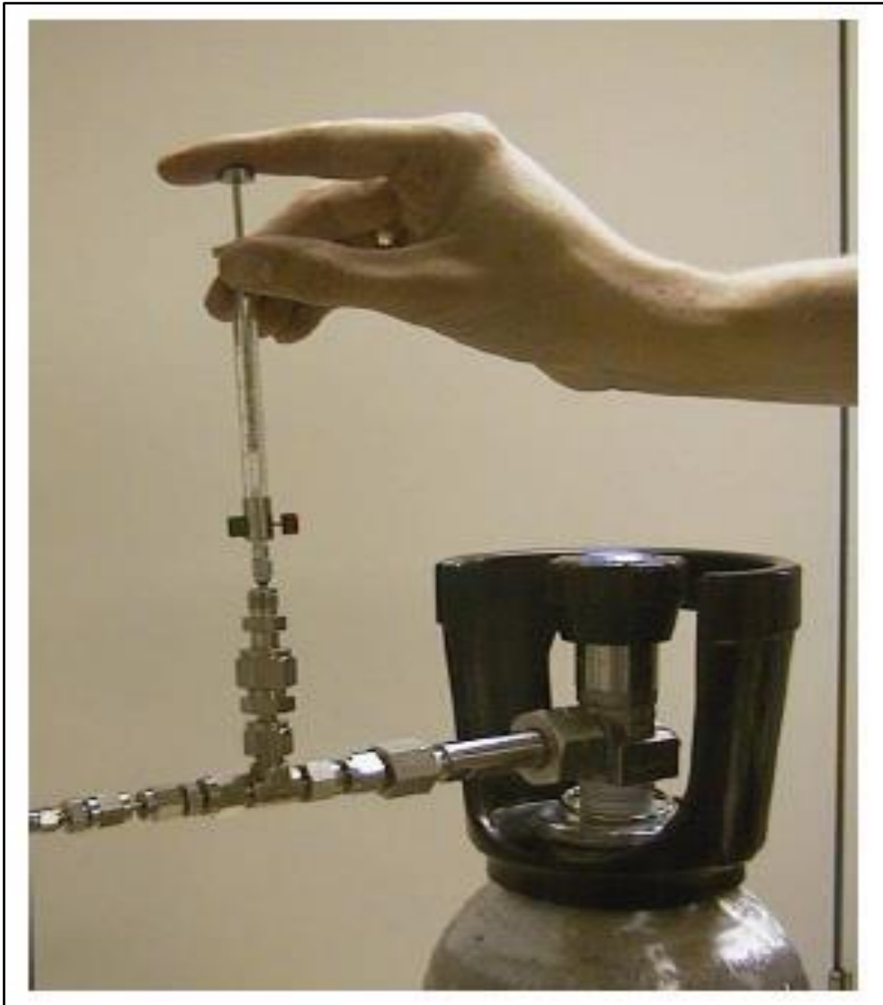
Figure 2-3: Introduction of liquid using the syringe method
