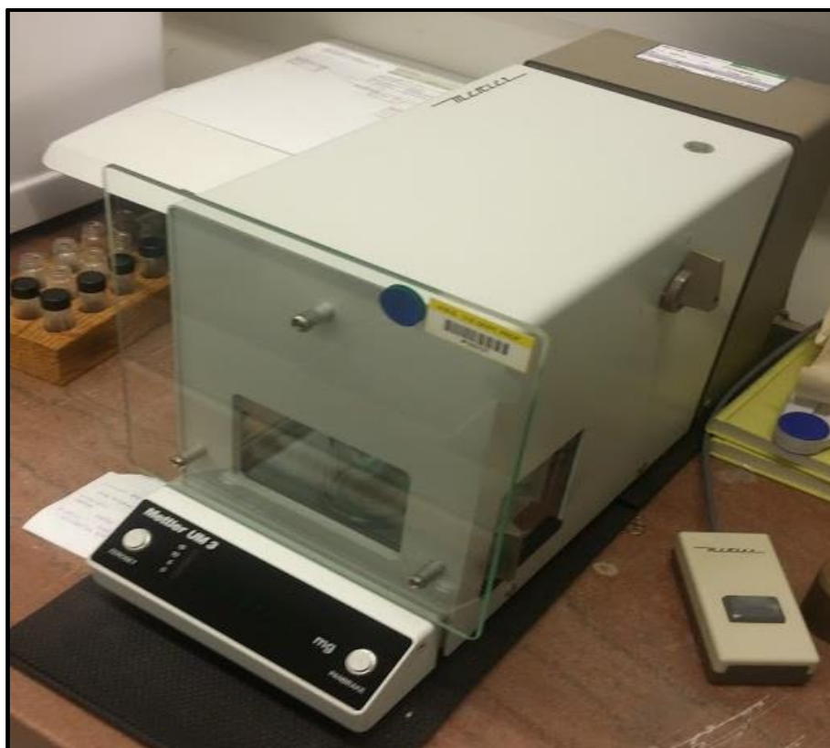
Figure 3-4: Weighing of capillary tubes on Mettler Toledo ultra-micro balance.
