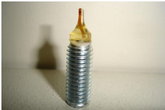
Figure 2.2. JB-4 embedded avocado root, mounted on a 10 mm steel bolt.
