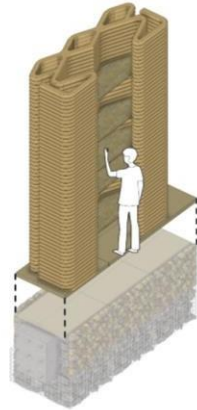
Figure 47: From coiling of pots to 3d printing of adobe walls (Author,2024).
