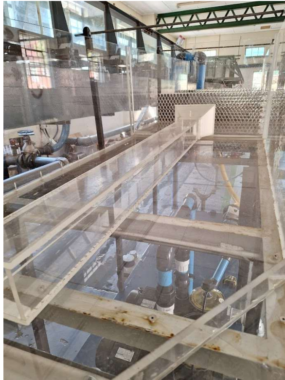
Figure 3-5: Culvert model from downstream side
