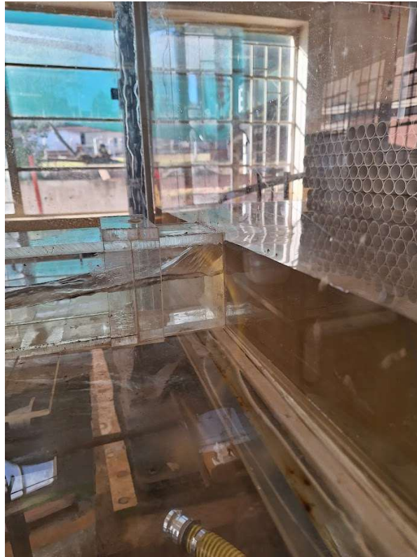
Figure 3-10: 90 degree headwall model with water flowing
