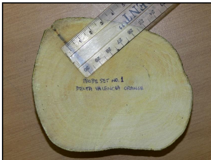
Figure 2.4. Measurement of the wounding width on a wood sample cut transversely from the trunk of one of the sample trees at the end of the measuring season in August 2009 (photo courtesy of Mark Gush).
