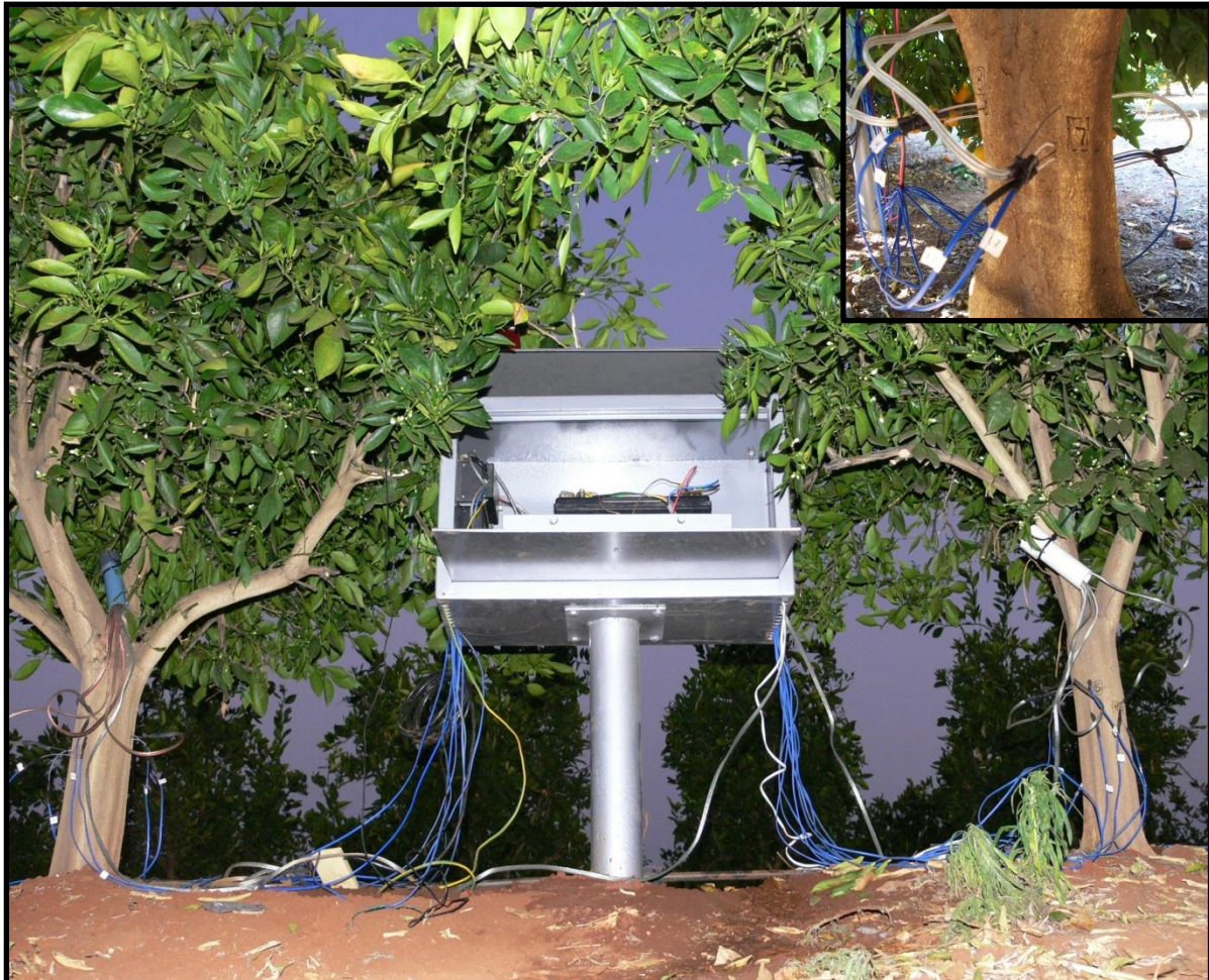
Figure 2.2. Sap flow probes installed in two trees in the 'Delta' Valencia orchard. Insert shows situation of the probes around a stem of one of the sample trees.
