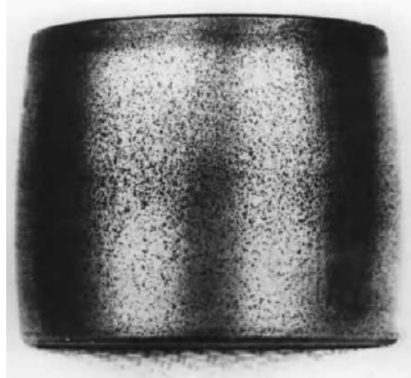
Figure 4: SEM micrograph of a hardened roller bearing after chemical wear (Bhushan, 2013: 360).
