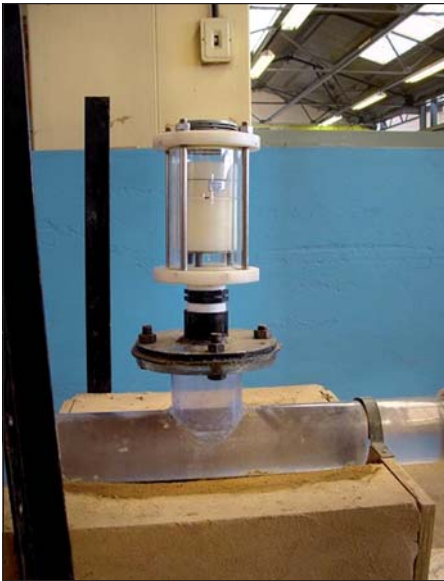
Figure 2 Discontinuity and air valve on 110 mm pipeline for Test 1 experimental setup
