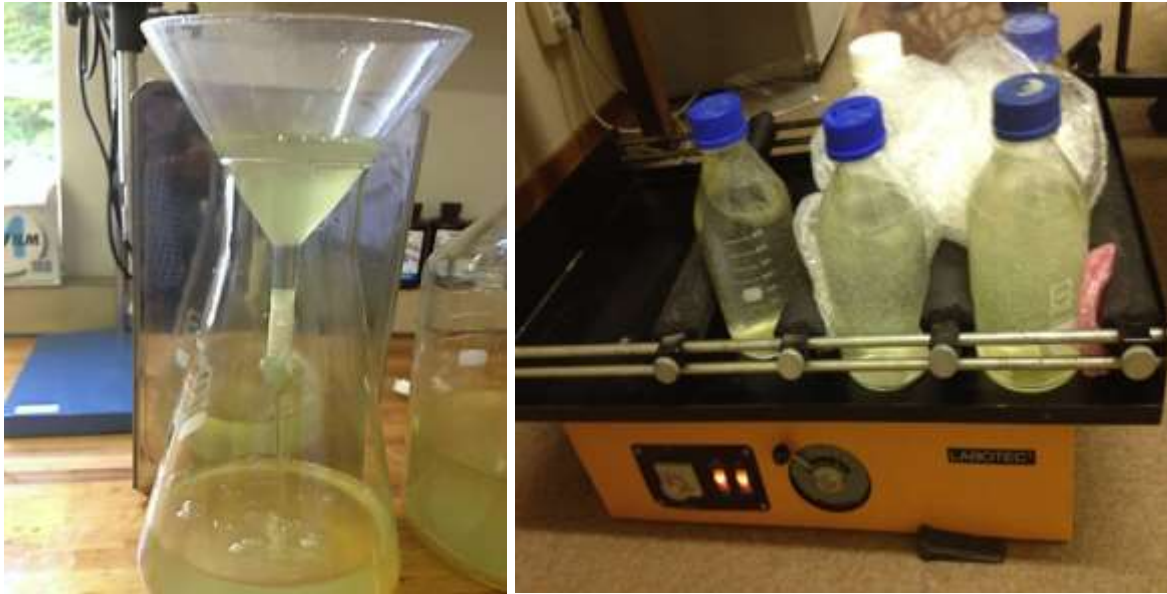
Figure 10 (left): Filtering of sonicated sample through nylon net (90- \mu\text{m} mesh size) to remove impurities.
