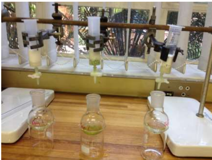
Figure 12: Methanol extraction process of microcystin from resin quantitatively transferred into a 25 ml Varian Bond-elute reservoir fitted with non-absorbent cotton wool.
