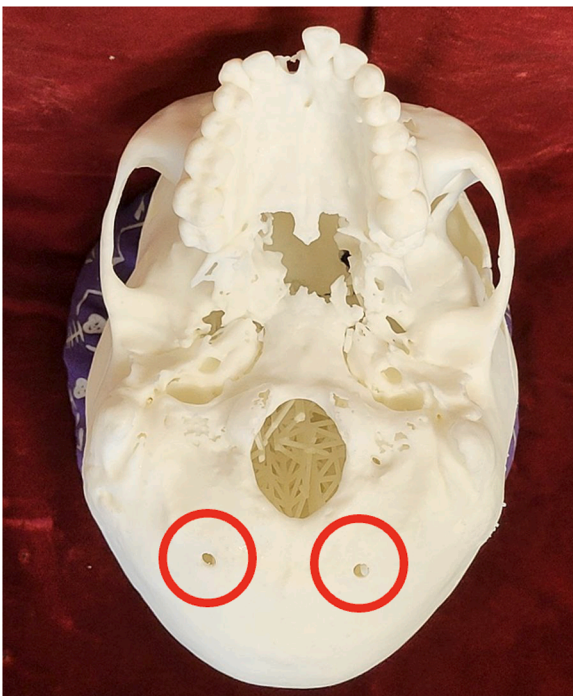
Fig. 4. Underside of the resin print of sample CR-01 showing the drainage holes circled in red.
