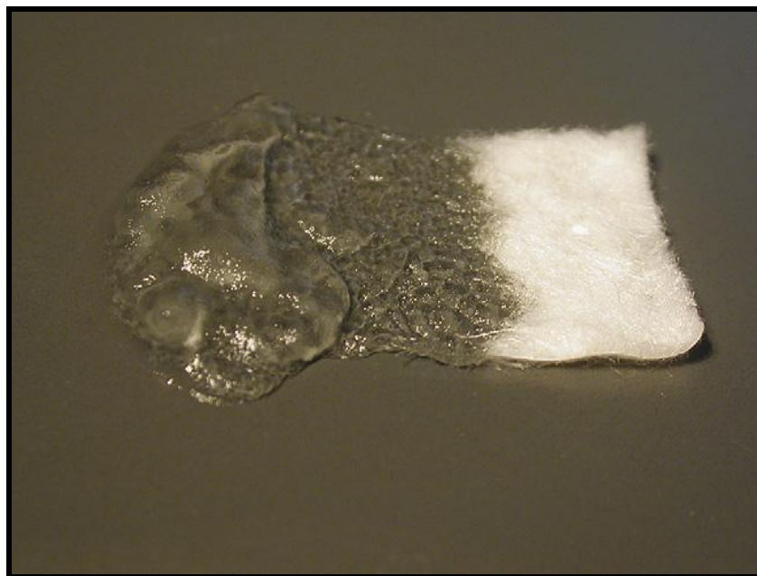
Figure 3. Hyaluronic acid gel formation when buffer is applied (Price et al. , 2007).
