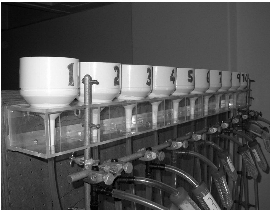
Figure 4.1: Angle view of the desorption measuring unit used to determine the desorption curves of several alternative casing materials and mixes. The desorption apparatus were based on system developed by Dr. Ralph Noble, from the Horticultural Research Institute, University of Warwick, UK. Notice that the bar is dropped and is not level with the Buchner funnel. This is to create a vacuum in the conical graduated test tubes for water to be removed from the saturated materials.
