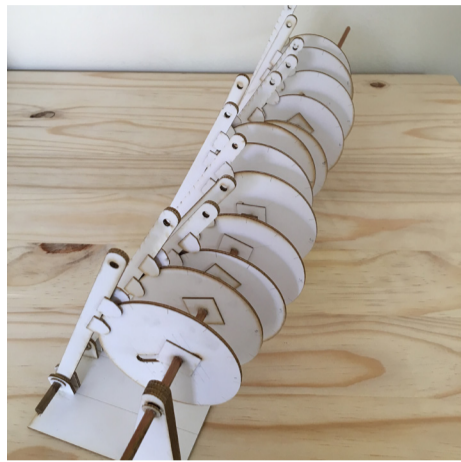
Figure 5.3.4 Kinetic mechanism with staggered cam and arm (Author. 2016)
