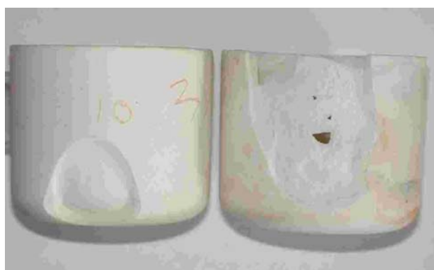
Figure 0-9: Cracking of alumina crucibles due to acid washing
