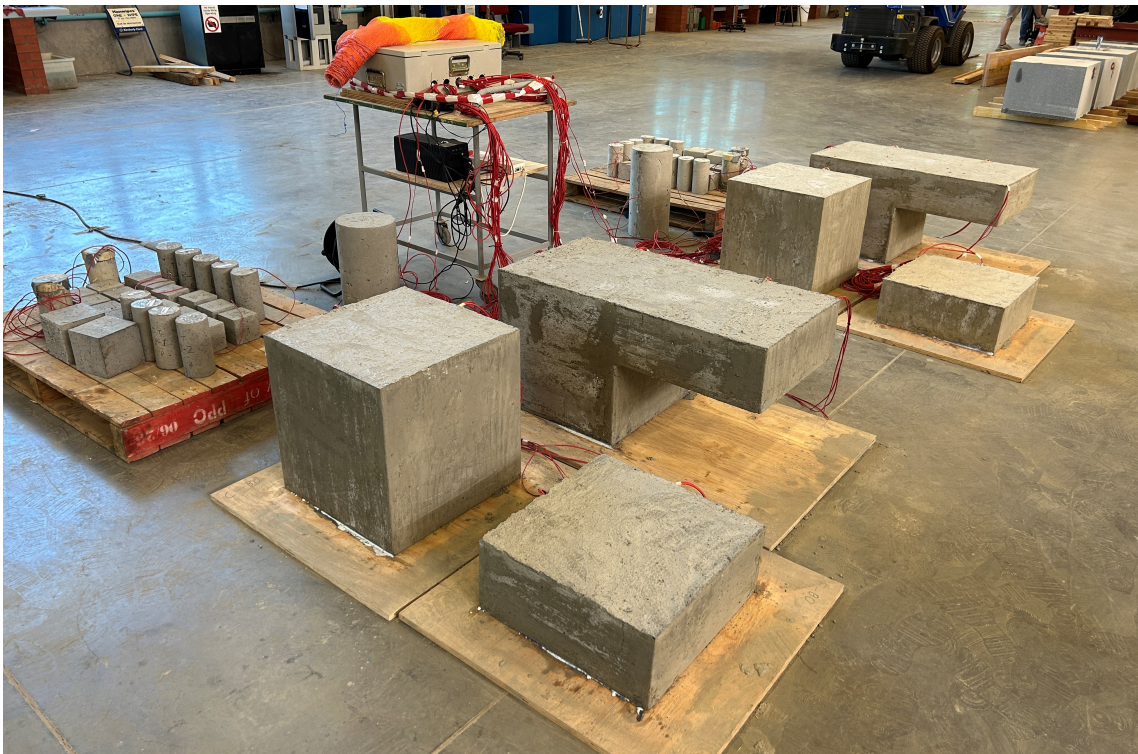
Figure 3.12: Casted concrete shapes and representative samples curing indoors on timber supports.
