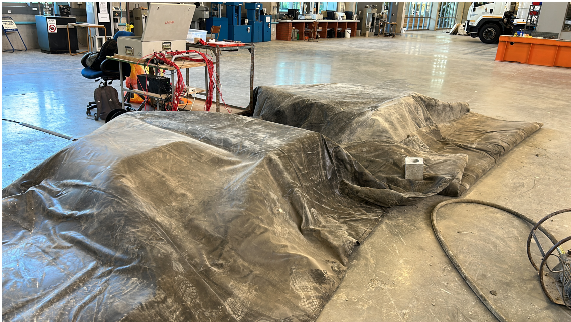
Figure 3.11: Casted concrete shapes and representative samples under curing blanket.
