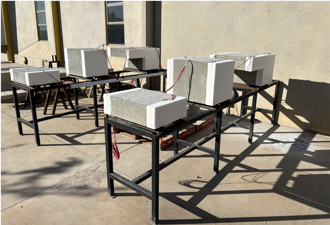
Figure 3.13: Outdoor placement of casted concrete shapes, and representative specimens.
