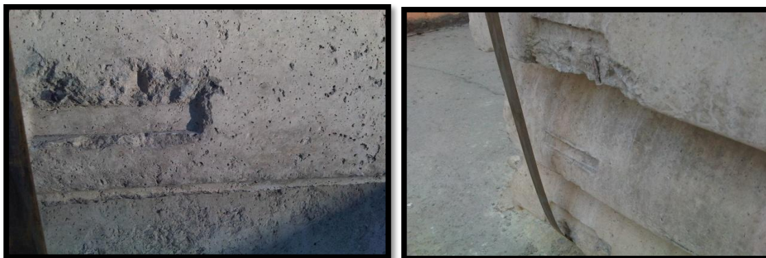
Figure 8: Defects caused by the handle part inside the mould.
