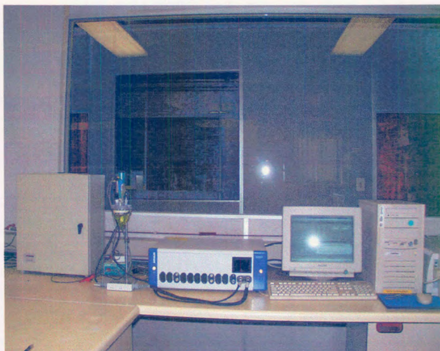
Figure 6.1 : An AutoLab PGStat 100 connected to a PC carrying the GPES
