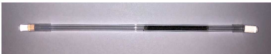
Figure 2.8: Graphene wool (GW) sampler showing the GW of 60 mm bed length housed in a glass tube.
