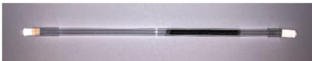
Figure S1: Graphene wool sampler showing the GW of 60 mm bed length housed in a glass tube with glass end caps held in place by Teflon sleeves. Source: Adapted from (Schoonraad and Forbes, 2019b).
