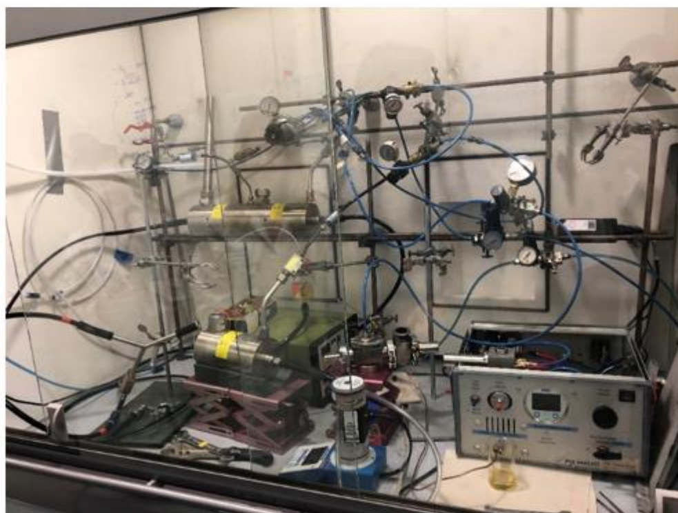
Figure S2: Photograph of the CAST generator sampling set-up.
