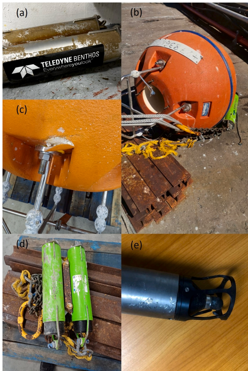
Fig. 3. (a) Trawled up acoustic releases from the Aliwal Shoal MPA acoustic mooring; (b-e) all trawled up components of the Child's Bank MPA acoustic mooring showing (c) damage on mooring float, (d) scrapped and scratched acoustic releases, and (e) damages on acoustic recorder.
