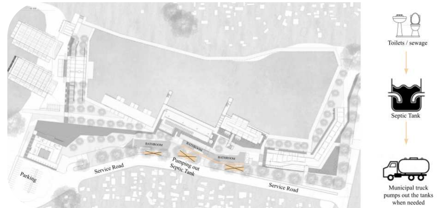
Figure 5.41: Illustrate the location of the conservancy tanks in the retained soil near the bathrooms for easy access to be pumped out by municipal sewage works (Author 2021).
