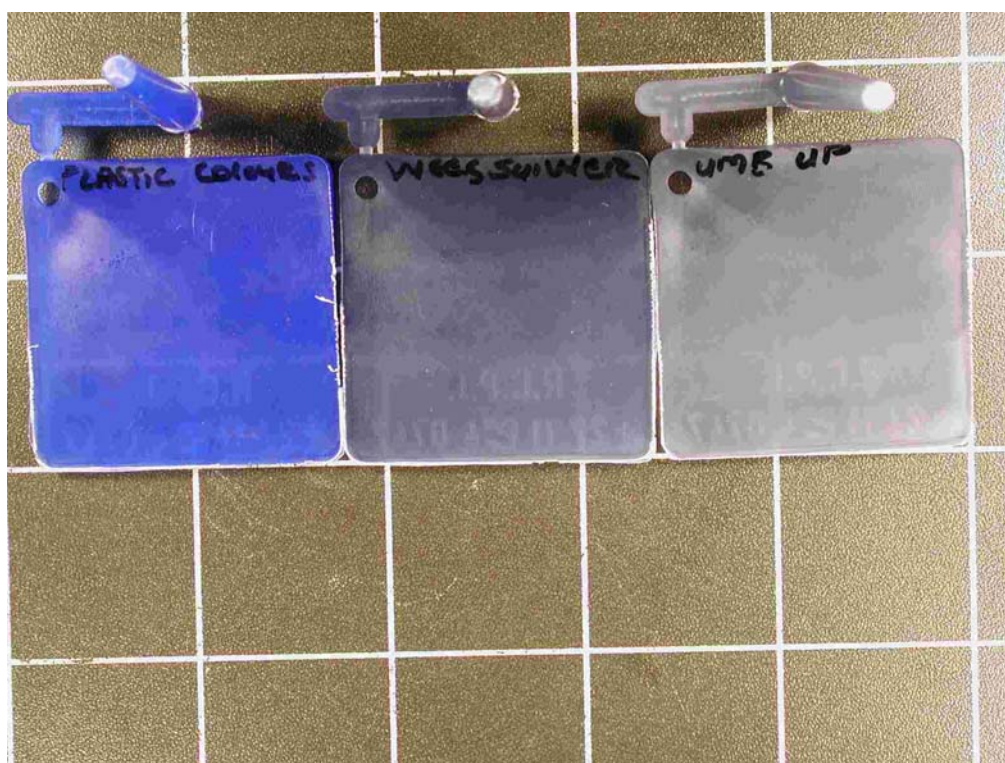
Figure 3-8: Plastic samples prepared with ultramarine products from this research and a commercial standard as pigments
