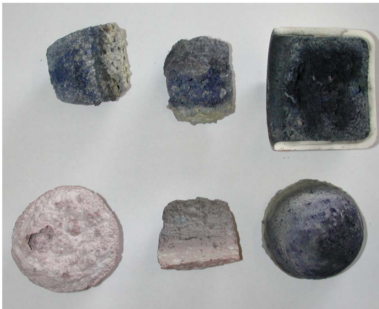
Figure 3-3: Agglomerated layered pigment cake formed during the synthesis of ultramarine blue, using fly ash as a starting reagent
