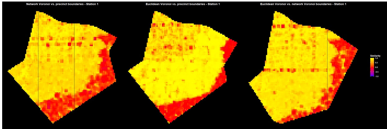
Figure 5.27: Police station A: Local similarity maps showing pixel-level agreement and differences between the networks of (i) Network Voronoi and administrative boundaries, (ii) Euclidean Voronoi and administrative boundaries, and (iii) Euclidean Voronoi and Network Voronoi boundaries.
