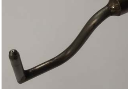
Figure 18: Tip of the five-hole pressure probe.
